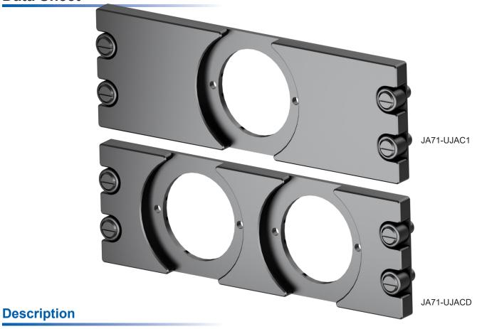
These two Dzus mount front panels are designed to accommodate either one or two of Jupiter Avionics' USB Chargers, UJAC-001 or UJAC2-001. Machined from 6061T6 aluminium and finished with a scratch resistant urethane paint, these plates are available in either black (FED-STD-37038) or gray (FED-STD-36321).
