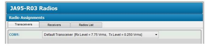
The Radios window is used to define the radios for the transceiver and receivers.
