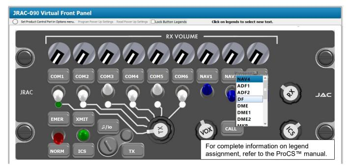
This Virtual Front Panel is used to define the 'names' associated with the control legends. The selected name will be used in all subsequent references to the associated transceiver/receiver, and will be used on the custom-generated Connector Maps and Interconnects. Also see section 2.6 (Virtual Control Panel).
