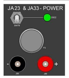
The **JA23 & JA33 - POWER** switch SW78 is a two-position, single pole toggle switch for power on/off. Annunciator DS22 will illuminate green when the unit is connected to a power supply and the switch is in the on (up) position.
