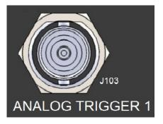
Three female panel-mount BNC connectors labelled **ANALOG TRIGGER 1** (J103), **ANALOG TRIGGER 2** (J104) and **ANALOG TRIGGER 3** (J105) are provided to interface with a signal generator.
