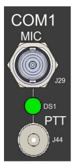
The **COM 1 MIC** is a black BNC female connector labelled J29. It is linked by a line to its associated annunciator DS1, and to a black single conductor panel mount banana jack marked **PTT** and labelled J44.
