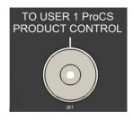
The **TO USER 1 ProCS PRODUCT CONTROL** connector J61 is a four contact 3.5 mm panel mounted jack.
