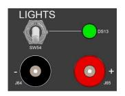
The **LIGHTS** switch (SW54) is a two-position, single pole toggle switch used for products with panel lights. When the switch is in the 'up' position, the lights will be on, and the annunciator DS13 will illuminate green. When the switch is in the 'down' position, the lights will be off and the annunciator will be dark.
