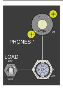
The **PHONES 1** section consists of a four conductor panel mount phones jack (J78) linked by a line to a female BNC panel mount connector (J89) and a single-pole two position toggle switch (SW76) labelled **LOAD**. The switch selects  $600\Omega$  in the up position and off in the down position.
