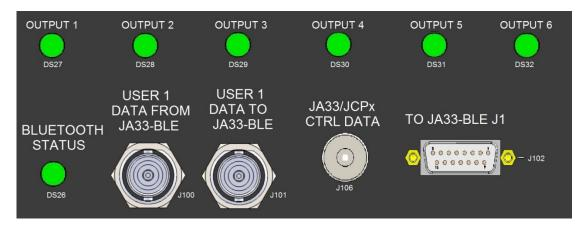
**OUTPUT** annunciators DS26 to DS32 Illuminate green when the associated output (**BLUETOOTH STATUS** and **OUTPUT 1** to **OUTPUT 6**) is active.
