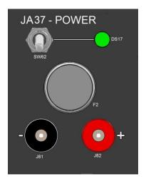
The **JA37 - POWER** switch (SW62) is a two-position, single pole toggle switch for power on/off. Annunciator DS17 will illuminate green when the unit is connected to a power supply and the switch is in the on (up) position.
