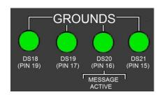
The **GROUNDS** annunciators DS18 to DS21 are marked with their associated pin numbers and will illuminate green when the relevant pin is grounded. DS20 (Pin 16) is linked by lines to the **MESSAGE ACTIVE** legend.
