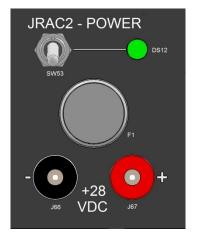
The **JRAC2 - POWER** switch (SW53) is a two-position, single pole toggle switch for power on/off. Annunciator DS12 will illuminate green when the unit is connected to a power supply and the switch is in the on (up) position.
