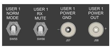
The **USER 1 NORM MODE** switch SW55 is a two position single pole toggle switch, used to select Normal mode when in the up position. The **USER 1 RX MUTE** switch SW56 is used to mute receive audio for USER 1.
