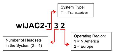
The **wiJAC2-T32** consists of up to three JB66-002 Wireless Aircraft Headset Adapters, and one JB67-002 Wireless Aircraft Intercom adapter.
