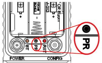
If either the JB67 or **any** of the JB66 units has been replaced, it will be necessary to re-pair **all** the units. This may also be necessary if either of the units has undergone maintenance.
