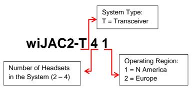
The **wiJAC2-T41** consists of up to four JB66-001 Wireless Aircraft Headset Adapters, and one JB67-001 Wireless Aircraft Intercom adapter.
